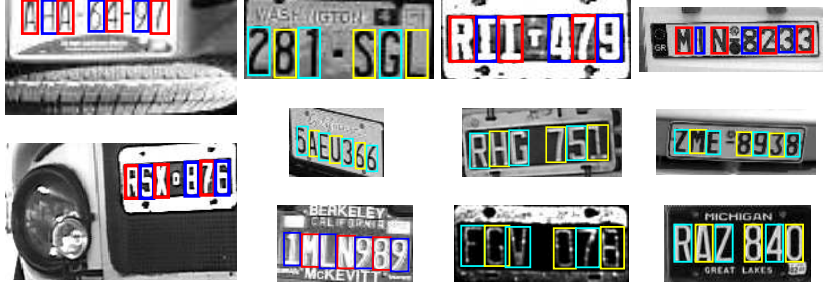
Fig. 3: Examples of character segmentation using char-grouping algorithm .
